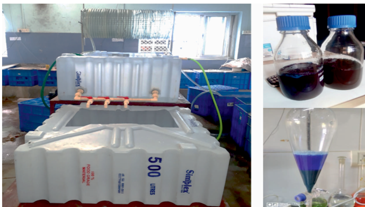
Fig. Prototype of indoor tubular bioreactor and Phycocyanin extracted from the biomass of S. platensis
