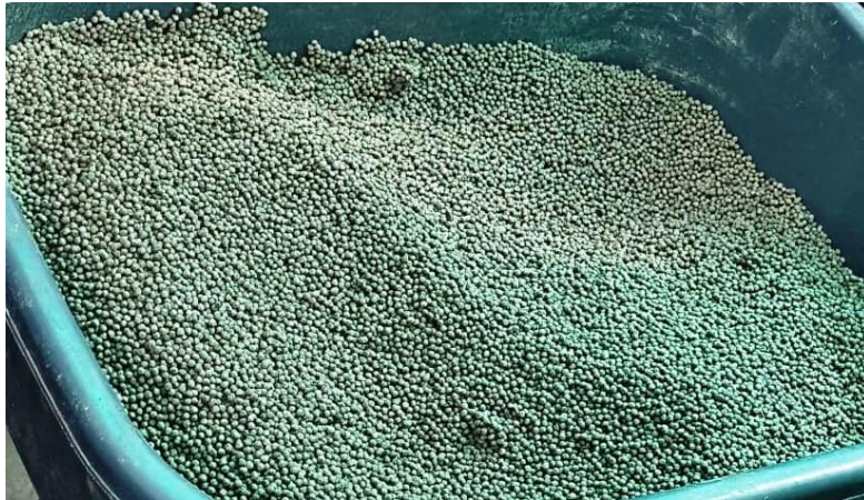
Fig 7: Sinking feed produced using twin screw extruder
