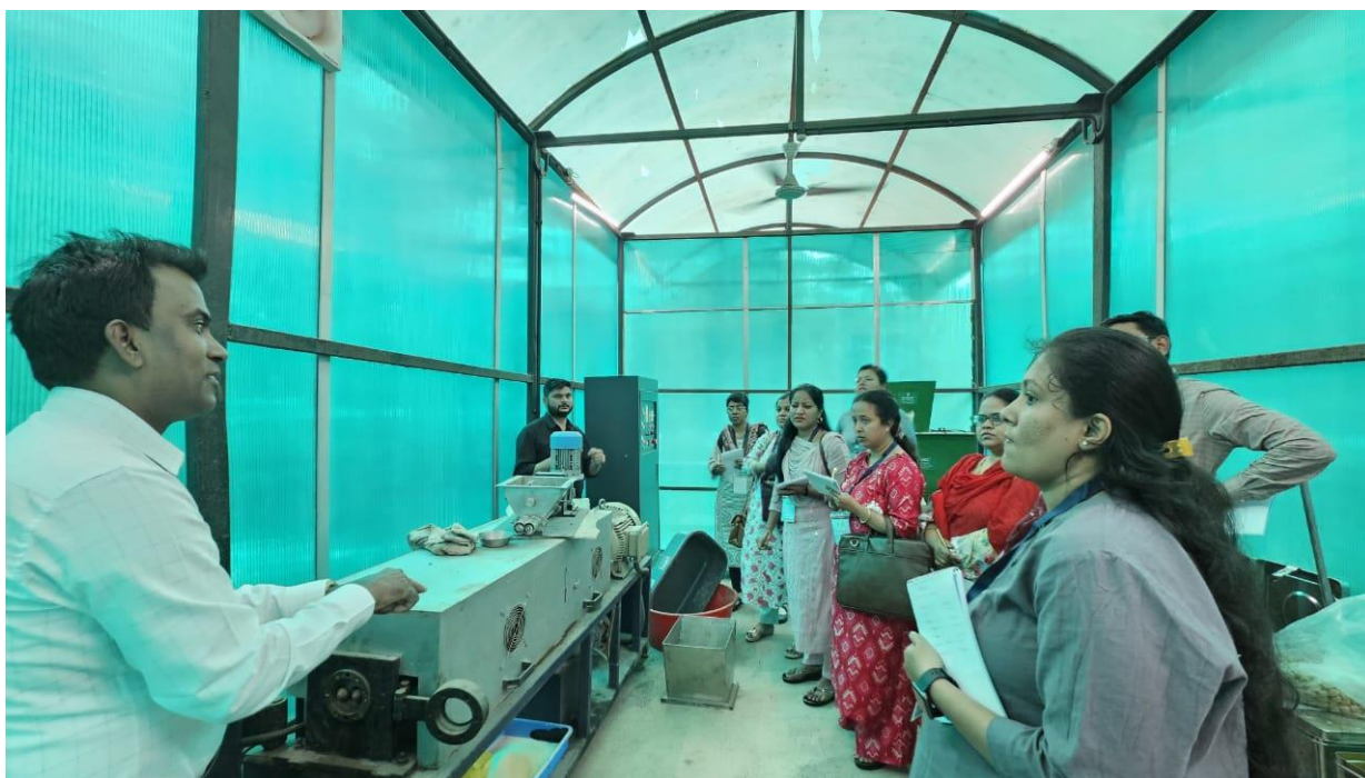
Fig. 5. Hands-on training on fish feed production using twin screw extruder
