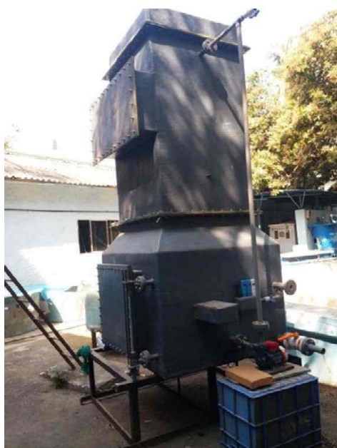
Prototypes of water filtration units (Capacity 1200-5000 L/h) r
