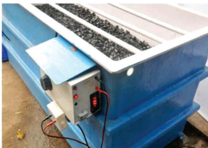
Electrically charged column based water filtration unit
