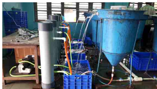
Recirculating aquaculture system for production of spawn
