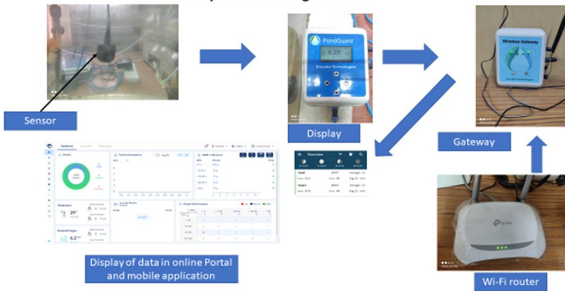
The flow diagram of retrieving the DO and temperature through sensors
