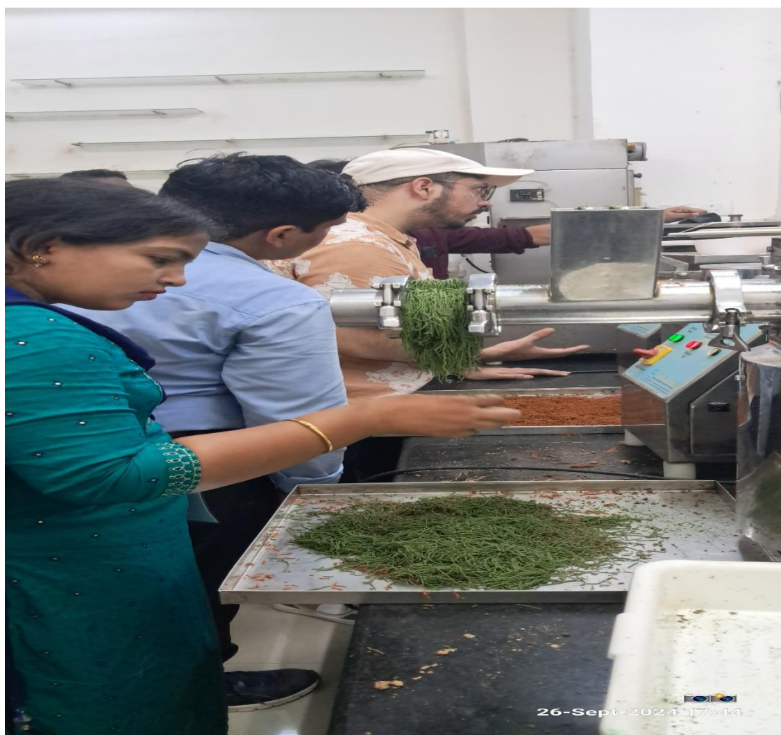
Fig 2: Production of feed using spheronizer by the trainees
