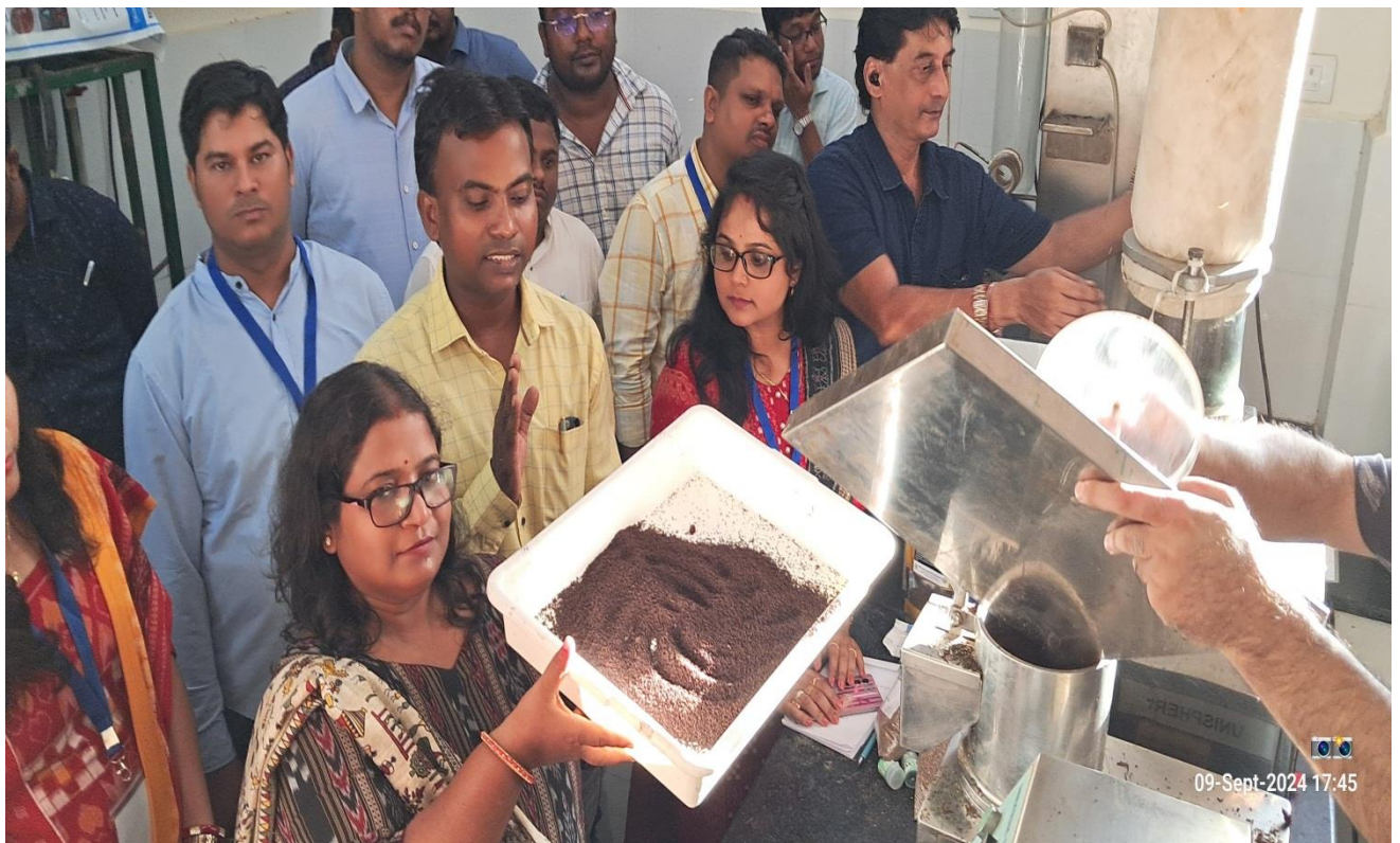
Fig 2: Production of feed using spheronizer by the trainees
