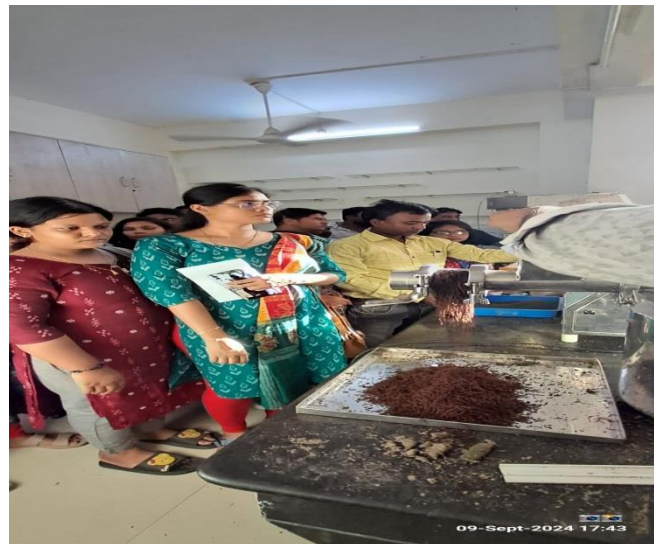
Fig 4: Production of feed using the single screw extruder by trainees
