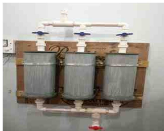
Wall Mounted Filtration Unit
