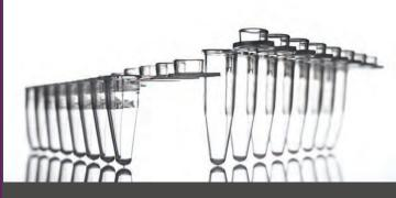
The tubes on each strip are joined together by three links to make the strip more rigid and help reduce any chance of spillage. The caps are flat and optically clear, enabling fluorescence to pass through without affecting the signal. Each cap is separately joined to a tube, making it impossible to either cross contaminate another tube with the wrong cap, or to lose a cap altogether.
