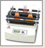
Benchtop shakers provide small capacity shaking for growth of biological organisms in your laboratory. This microprocessor controlled shaker offers a number of advanced features including userfriendly digital set points keypad, electronic timer 1 minute to 500 hours, non-volatile memory and alarm programmed to indicate when timer operation has expired. The shakers are reliable and affordable, compact yet without compromise.
