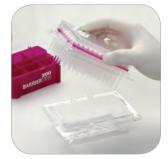
Remove alignment plate from the packaging base by gripping alignment plate using the upper portion of the clamshell packaging.
