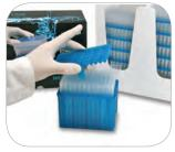
Squeeze the side posts of the alignment plate and pull up to disengage from the insert card.
