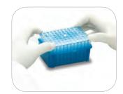
Secure plate by firmly pressing on all four corners of the alignment plate.
