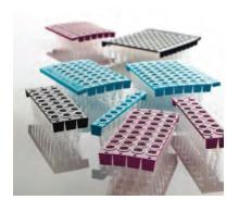
Frame Colour options Well Colour options Clear or White Other options Black frame with white wells · 2D barcoding MAX = 300ul WORKING = 250ul Rigid PCR plate that can be divided into smaller plate sections and strips Easy to break at any temperature End tabs for easy handling and labelling Numbered strips prevent sample errors 2-component design prevents distortion and evaporation
