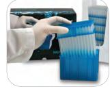
Hold the alignment card away from the side posts and insert the tips into your empty tray.
