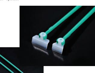
Scar<sup>™</sup> Scratcher improves the uniformity and reproducibility of the possible products used in cancer metastasis, wound healing and cell migration research. Scar<sup>™</sup> Scratcher consists of a Lid with holes and a Scratcher, in 6 or 24 well format.
