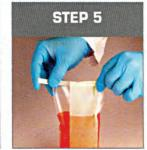
Fold both wire ends onto the bag to provide air-tight and leak-proof closure.
