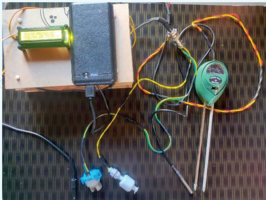
Fig 1: IoT prototype for Biofloc Fish Culture
